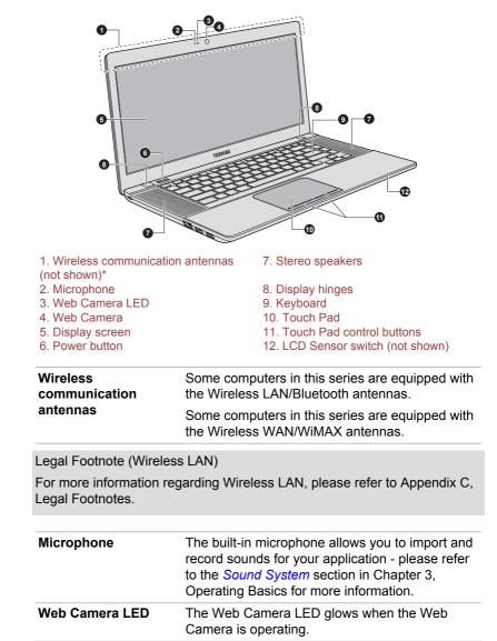
Figure 2-5 The front of the computer with the display panel open
